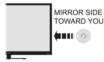
Do not force the disc into the mechanism, the loader should take the disc when inserted partway.
